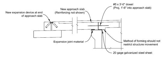
Figure 33-3: Expansion Joint Relocation
