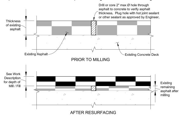
Figure 33-1: Asphalt Thickness Verification Detail
