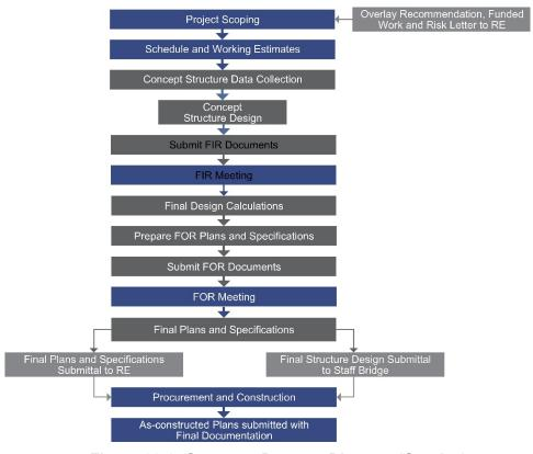
Figure 33-6: Structure Process Diagram (Overlay)
