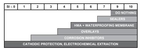
Figure 33-2: Optimal Corrosion Control Based on Susceptibility Index
