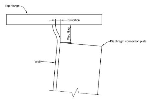
Figure 33-5: Web Gap Distortion
